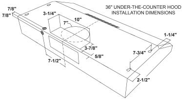
Exhaust outlet connects to 3-1/4" x 10" rectangular duct. Vent top or rear. Includes rectangular damper.
